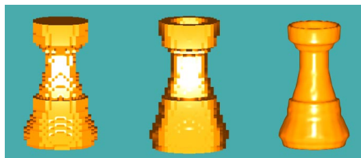
Figure 2: Rendering of rook voxelised using (a) 1 regular sample, (b) 7 \times 7 \times 7 regular samples, (c) distance shell
