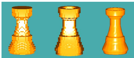
Figure 1. Rendering of rook voxelised using (a) 1 regular sample, (b) 7 \times 7 \times 7 regular samples (Section 3.1), (c) distance shell
