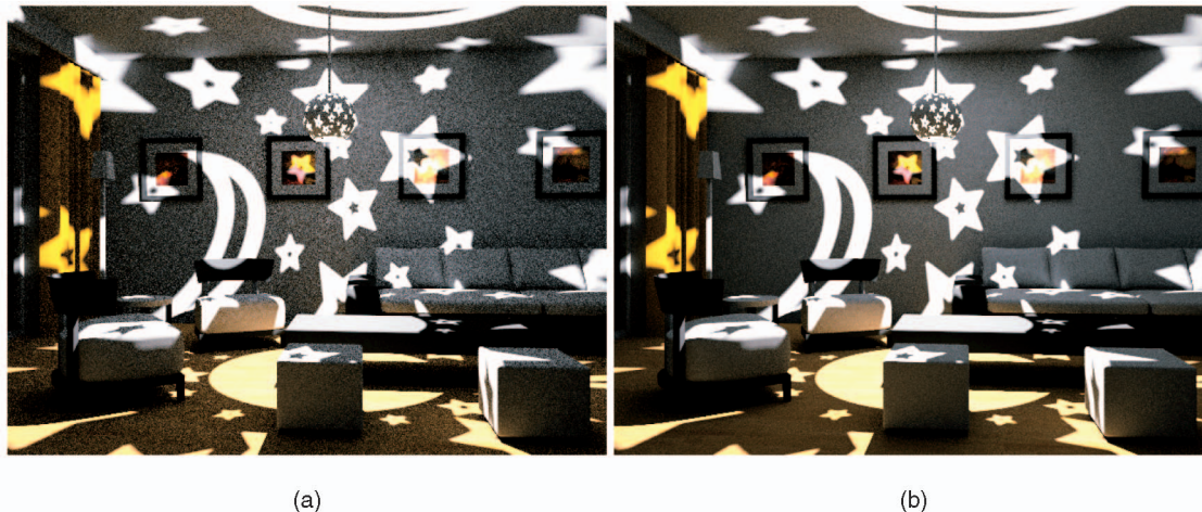
Fig. 13. Living Room with Lantern. 640 \times 480 pixels. 50 FGRs per pixel. 576K photons (50 in the radiance estimate). (a) Conventional photon mapping. (b) Hierarchical photon mapping.
