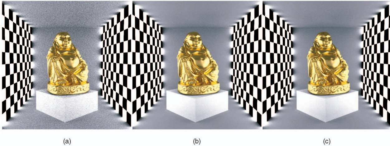
Fig. 11. Cornell Box with Glossy Buddha. 600 \times 600 pixels. 414K photons (50 in the radiance estimate). (a) Conventional photon mapping, 50 FGRs per pixel. (b) Hierarchical photon mapping, 50 FGRs per pixel. (c) Conventional photon mapping, 300 FGRs per pixel (same visual quality as (b)).
