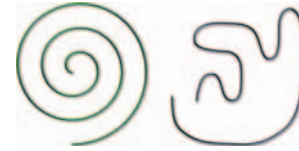
Fig. 2. Both of these curves exhibit very similar curvature magnitude values. Therefore, a single global measure fails to distinguish streamline sufficiently. In this case, the tortuosity attribute would fair better but there are cases where this would also fail. A better method creates a distinctive signature for the streamlines using density-based attributes.
